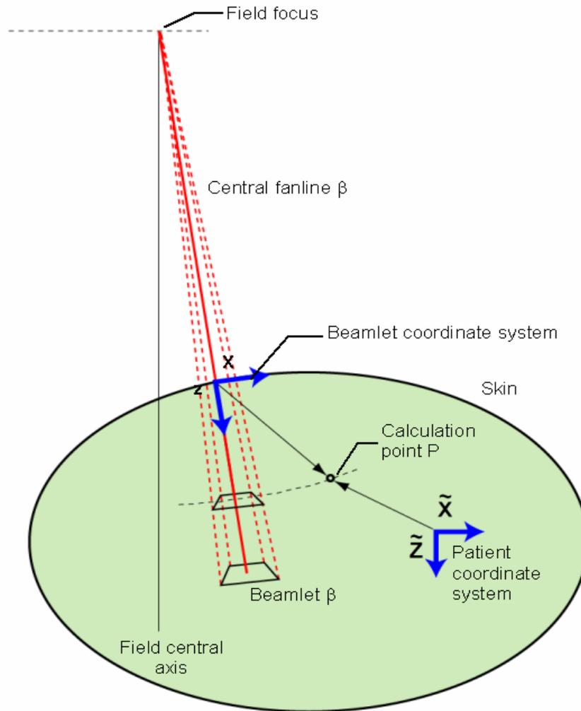
**Figure 5: Coordinates in patient coordinate system and beamlet coordinate system on X–Z plane.**
