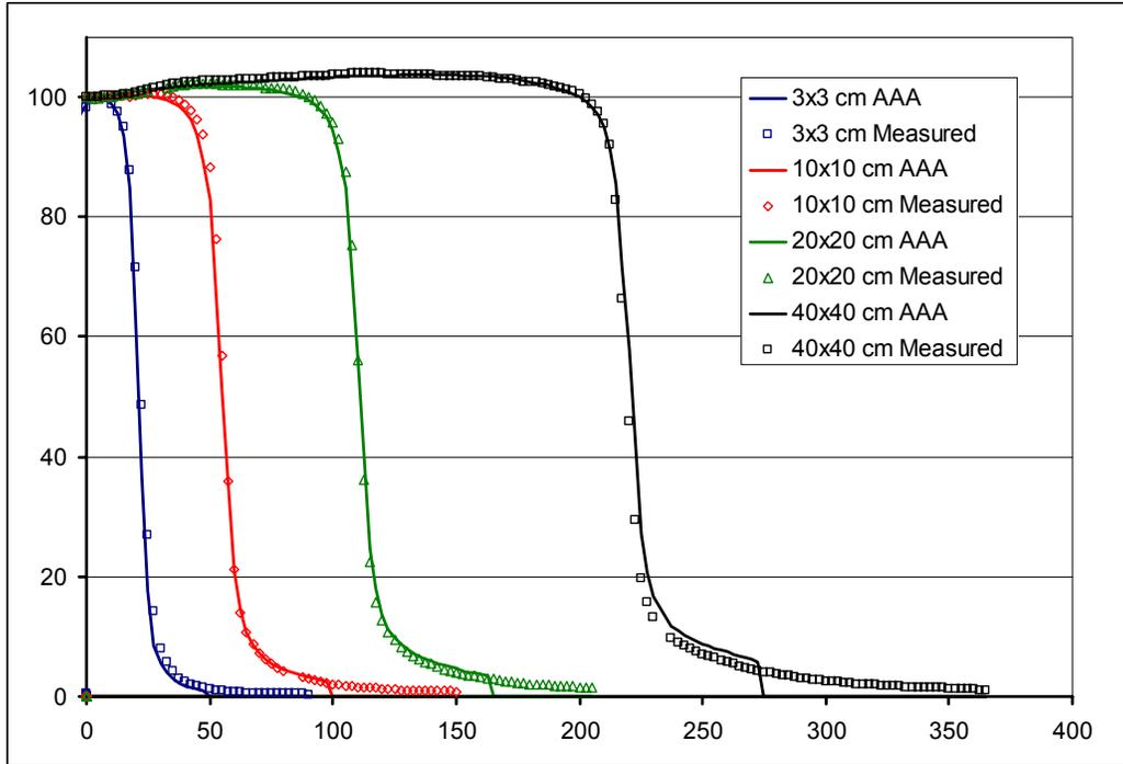
**Figure 11: Profiles for depth 10 cm for 18 MV**
