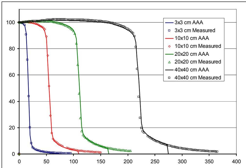
**Figure 8: Profiles for depth 10 cm for 6 MV**
