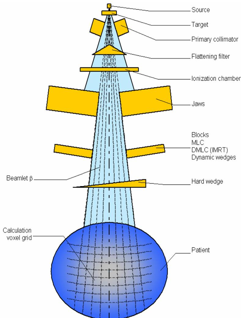
**Figure 4: Treatment unit components, broad beam division.**
