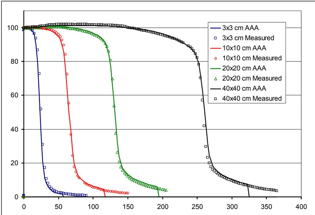
**Figure 12: Profiles for depth 30 cm for 18 MV**
