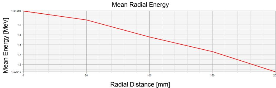
**Figure 2: Example of the mean energy as a function of distance from the beam central axis of a 6 MV photon beam.**
