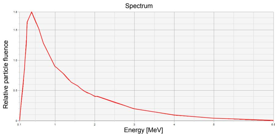
**Figure 1: Example of a 6 MV photon spectrum.**
